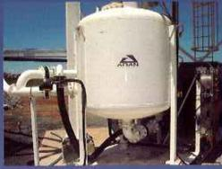
Bulk Cement Storage silos and Aran APTS dense phase pneumatic transfer system, all integrated with the plant control system. Bulker bag handling systems available.
